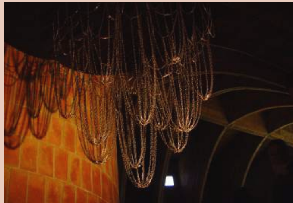
Gaudí's upside-down genius, the catenary string model revealed how gravity itself could sketch the perfect arch.
